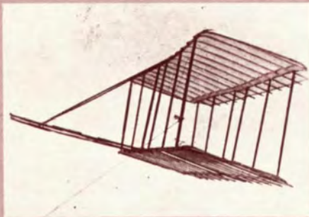
The Wright Brothers' first airframe was the 1900 glider, here being flown as a kite.
