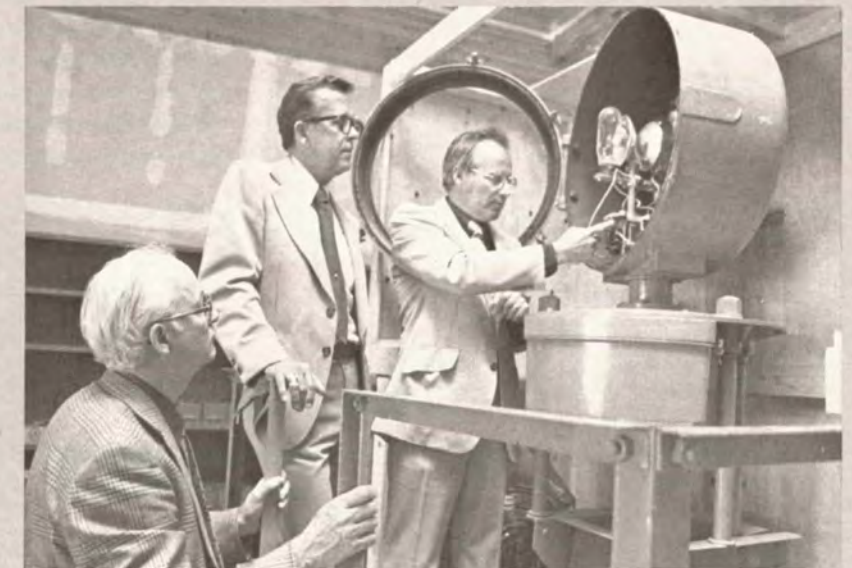
RESTOCKING HISTORY —John Tompkins (right), San Diego AF Sector manager, shows Western Region AF Division chief Bob Frehse the automatic lamp transfer mechanism of an Airway Beacon Light being donated to the San Diego Aero-Space Museum, which was destroyed by fire earlier this year. With the help of groups like Western Region FAAers, the museum will be reopened December 17, the anniversary of the Wright Brothers' flight. Looking on is San Diego Sector technical support officer Ed Hutchinson.
