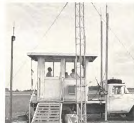
This air-conditioned temporary tower mounted on a flat-bed at the Opa Locka, Fla., Airport is a sturdier structure for regular use around the region.
