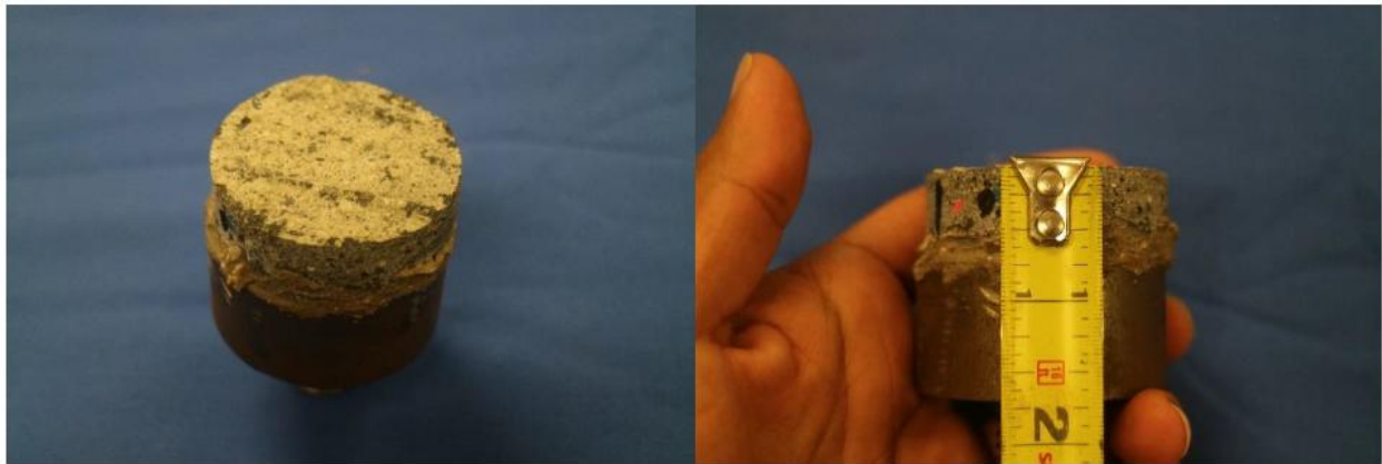
Figure 6.30. Core sample No. 6 from pull-off testing on the bridge (UHPC Phase V, Figure 6.101)
