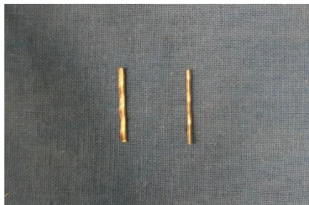
Figure 6.23. Previously utilized Steel Fiber - U vs. Modified Steel Fiber - U (UHPC Phase V, Figure 4.5)
