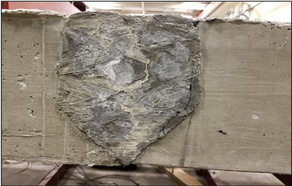
Figure 6.6. Specimen No. 2 - initial separation at bond point; (UHPC Phase IV, Figure 5.59)
