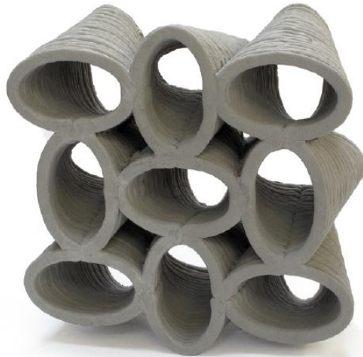
Figure 7.13. CAD model for the multifunctional wall and the 3DP-UHPC multifunctional wall
