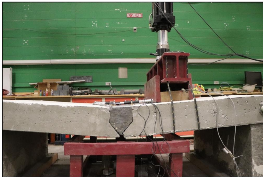
Figure 6.8. Specimen N0. 4 - failure of system; (UHPC Phase IV, Figure 5.87)
