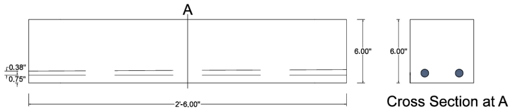
Figure 6.18. NSC beam design with reinforcement (UHPC Phase IV, Figure 5.159)
