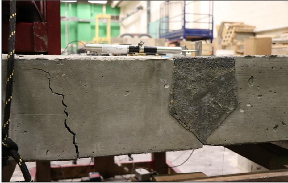
Figure 6.5. Specimen No. 1 - failure at north face; (UHPC Phase IV, Figure 5.38)
