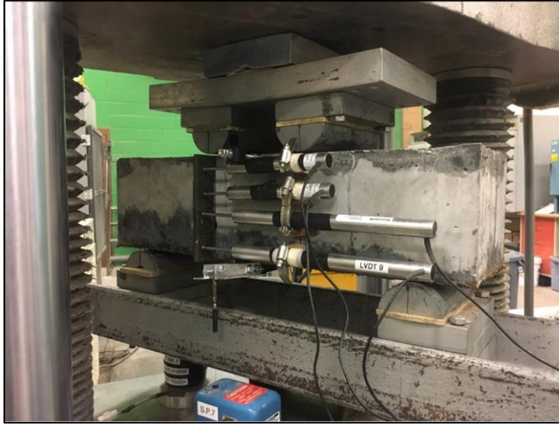
Figure 6.20. Test set up for beams with 1 in. of UHPC at the bottom and at the top (UHPC Phase IV, Figure 5.165)
