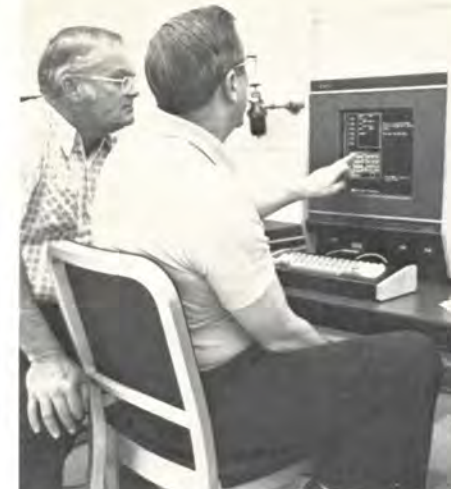
In the FAA Academy's Flight Standards Airspace and Procedures Section, instructor Joe Reddin (left) monitors the use of a Plato V display under evaluation, which duplicates the RNAV computer in flight inspection airplanes. Battle Creek, Mich., FIFO pilot Leo Blakely punches the buttons.
