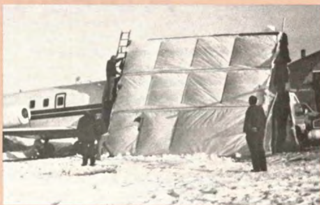
INGENUITY —When maintenance technicians from the Aeronautical Center's Aircraft Services Base had to repair a damaged FAA Sabreliner in the winter cold of International Falls, Minn., they found no hangar space available. To fend off the 35-degrees-below-zero chill, they built a hangar around the nose and nosewheel made of wood framing and plastic, equipped it with electricity and heat, and got the repair job done comfortably.
