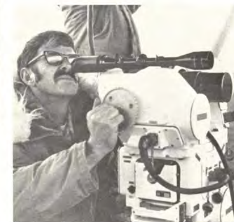
At Charleroi Airport near Brussels, Belgium, J. J. Collins operates a theodolite under the azimuth antenna to confirm the accuracy of demonstration flights by the agency's Convair 880 and Boeing 727.
