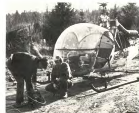
Safety in the air is partly dependent on the emergency release in the circular rings between the chopper cable and the load. Inspector Butterworth watches as a pilot checks the release mechanism.
