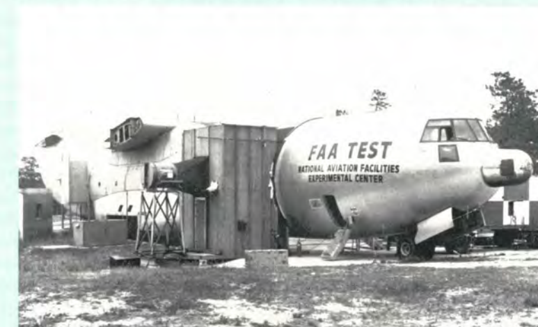
SAFETY FIRST —NAFEC is conducting fire tests in this C-133 transport whose interior has been modified to resemble that of wide-body jets. The effects of heat, smoke and gases in the passenger cabin from fuel fires are being studied to find means to reduce fatalities in aircraft accidents.
