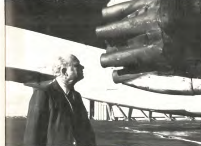
Seattle operations inspector Ed Gremmer checks over one of the jet-engine tailpipes during a B-707 preflight inspection. It's not a post-flight check for flak damage!
