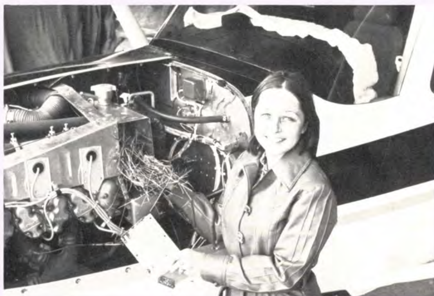
FOR THE BIRDS— Phyllis Harrington, Lebanon, N.H., Tower controller, spotted birds flying in and out of the cowling of a Cessna 172 that had been parked at the airport only a few hours. A local A&P mechanic pulled out this nest from the plane's oil cooler.
