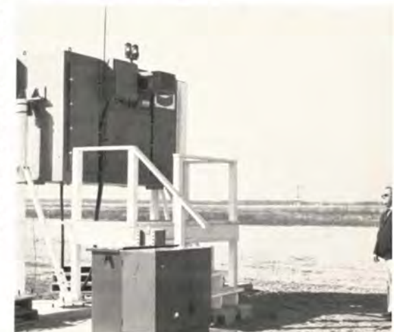
As part of a daily inspection of Atlantic City Airport's landing and navigation aids and specially installed NAFEC equipment, airport operations specialist Jack DeStefano checks out a microwave landing unit.
