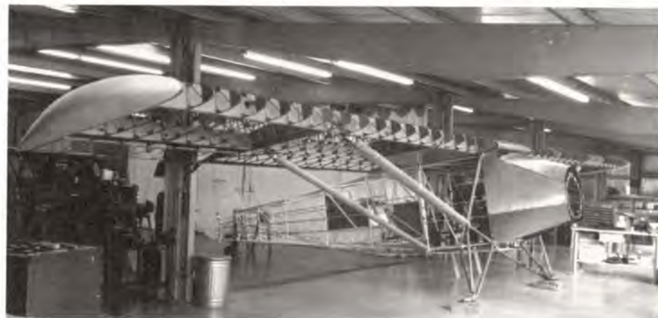
The "Spirit of St. Louis," vintage 1977, takes shape in the museum shop of the Experimental Aircraft Association. Here, the control surfaces were installed temporarily for fitting and adjustment.
