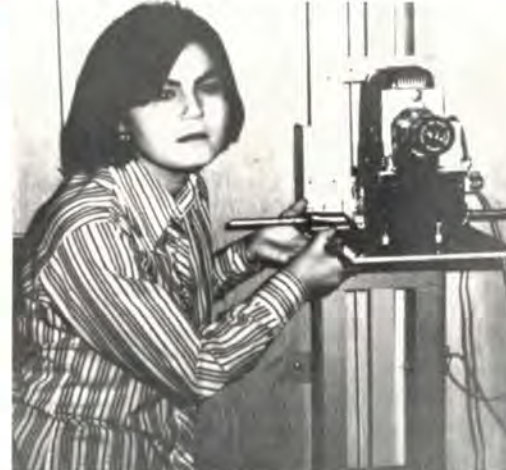
Fontaine Young, CAMI anthropologist, operates the photoanthropometer, which is used to measure pre-schoolers' body structure prior to mapping.
