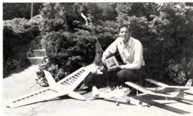
RC glider, biplane and trainers are among John Reynolds' fleet. Pennants on transmitter antenna identify its frequency. (Top) RC plane's fuselage is packed with motor and (left to right) batteries, motor speed control, with receiver underneath, and control pushrod servos.
