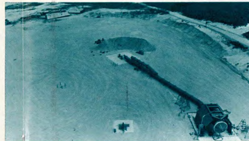
BIG WIND —This is the new Air Blast Test Facility at NAFEC. George Chamberlain, Paul Boris, Tony Spezio and Charles Cole are working here on a variety of projects for fire-testing engines and small components and testing fire extinguishers, fire detectors and aviation fluids. The airspeed at the test stand can exceed 300 knots.
