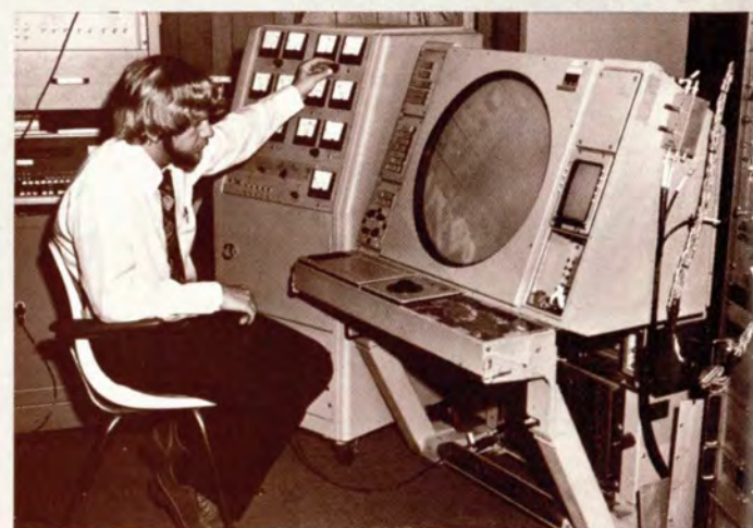
PVD DOCTOR —John Aschenbach adjusts a new cathode-ray-tube tester that he and Phil Gustafson developed at NAFEC for testing plan view displays for ARTCCs. It checks the tube and the circuitry and can be modified for terminals.
