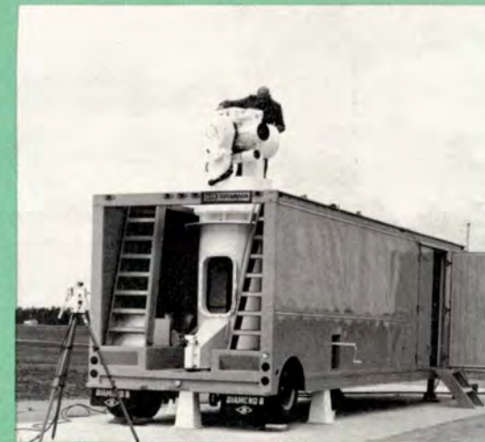
MLS TRACKER —NAFEC technician Paul Blumenauer checks over a new laser tracker that is capable of plotting the accuracy of an airplane that is testing microwave landing systems and other guidance equipment.
