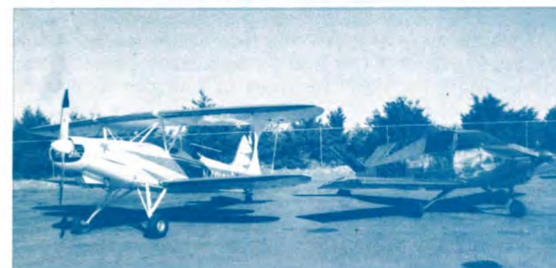
PLANE BUILDERS, TOO —A pair of Goodland, Kan., FSS specialists have built their own aircraft. The "Starduster Too" biplane, built by Edward Middleton and his father, sports a 150-hp Lycoming with full inverted fuel and oil systems. The all-metal "Davis DA2A", built by facility chief James Waddell and his friend Phay Hussey, has a Continental A-65 but is slated to get a C-85 engine eventually.
