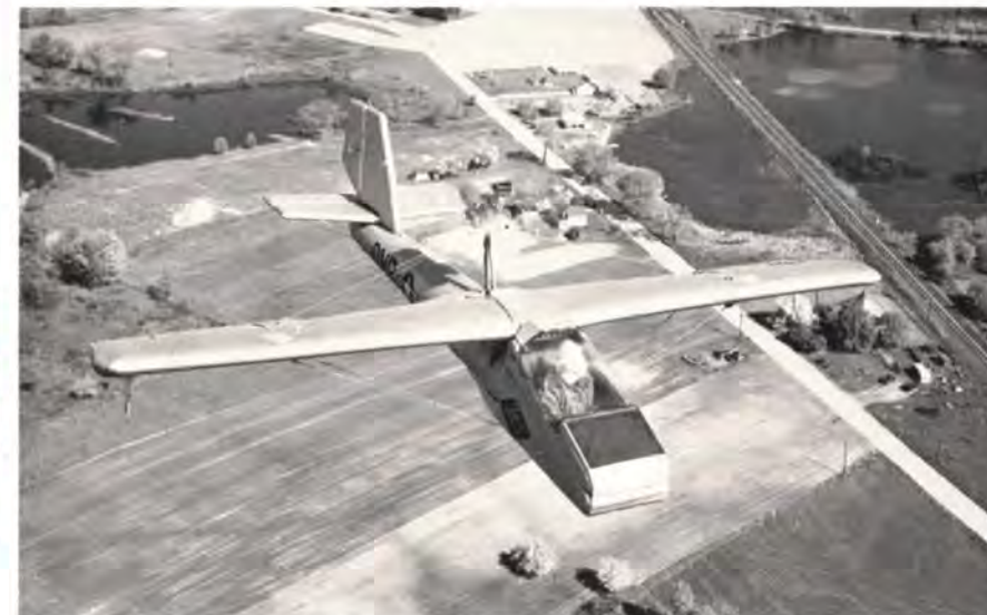
The Inflatoplane was a real innovation. The pilot just blew the thing up, hopped in and went for a spin, zipping along at 74 miles an hour at up to 10,000 feet.
