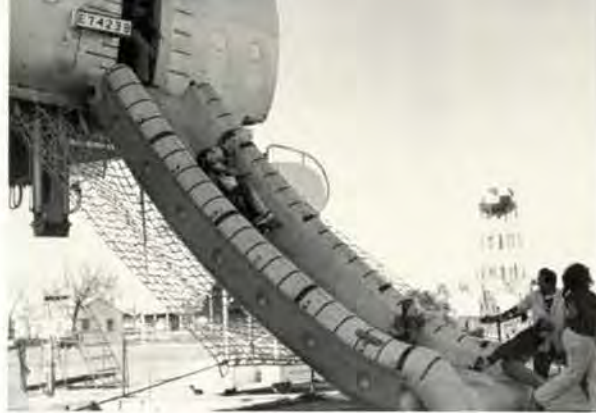
The Civil Aeromedical Institute continued its protection and survival studies in 1975, including tests of the emergency evacuation of the handicapped via slide from the evacuation simulator. Actual handicapped persons weren't used in this test.
