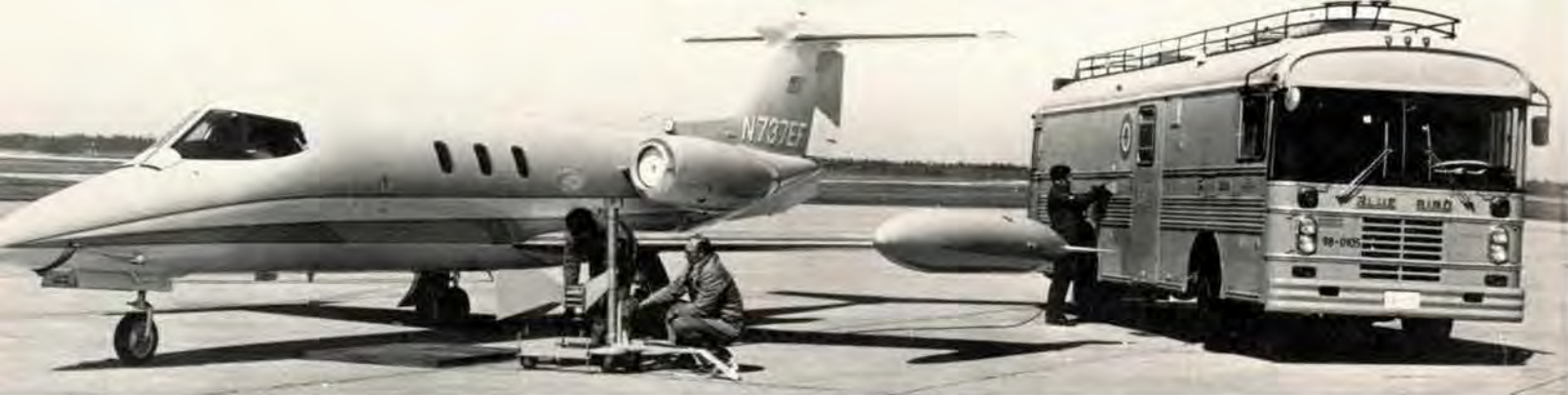
Technicians aim a horn antenna at a plane's beacon antenna in a test using a system housed in the van to check out transponder performance. It was demonstrated for the first time at the Reading Air Show in 1975.
