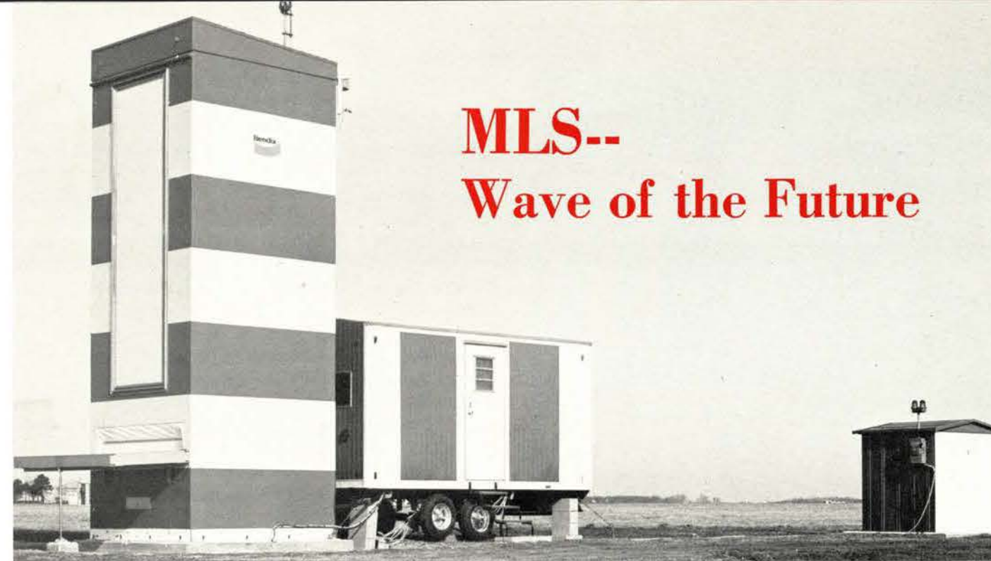
NAFEC is testing MLS scanning-beam equipment, which requires three sites along the runway. This is the glide-slope equipment, consisting of (from the left) an antenna, an equipment shelter and a power transformer.
