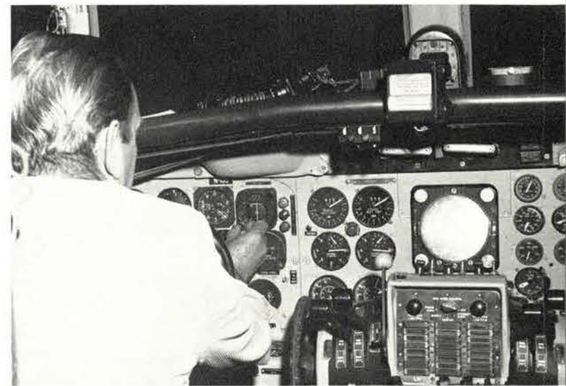
NAFEC test pilot John Ryan adjusts his ILS-VOR cross-pointer display that can be switched for MLS or ILS.
