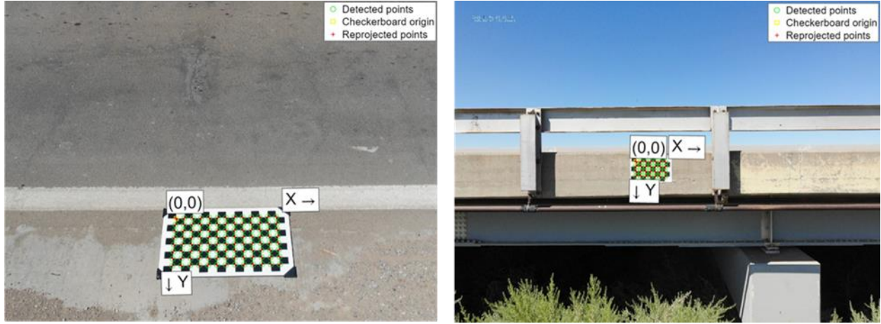
Figure 20. On-site camera calibration examples for the second bridge (NBI bridge number: 06255)
