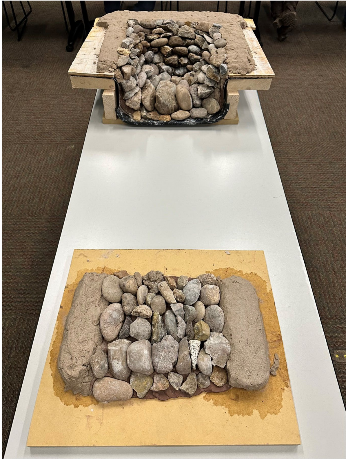
Figure 4-2. Prototype desktop model of a Zuni Bowl and One Rock Dam built by RGR.
