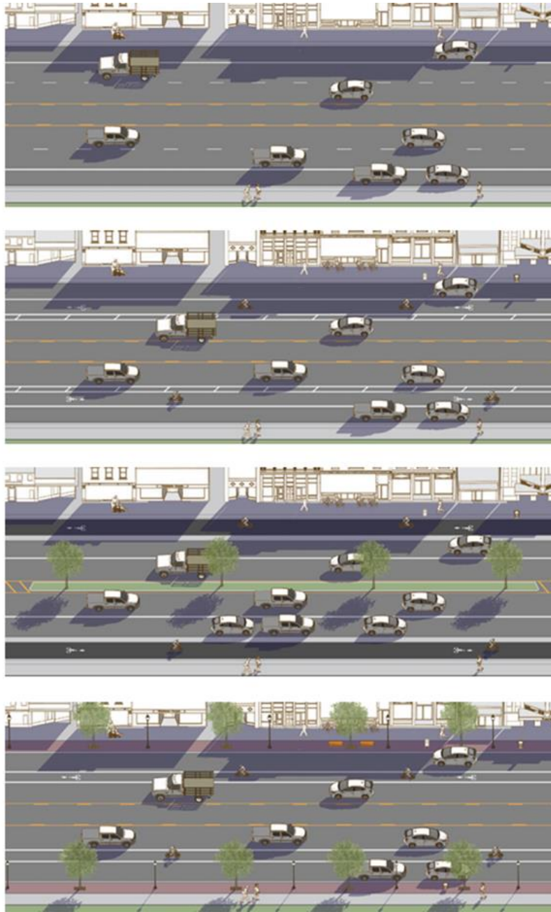
FIGURE 1. Example of five-lane Main Street (top picture) conversions to Road Diet with Bike Lanes (2nd from top); Median and Separated Bike Lanes (3rd); Streetscape Expansion with Bike Lanes (bottom). (8)
