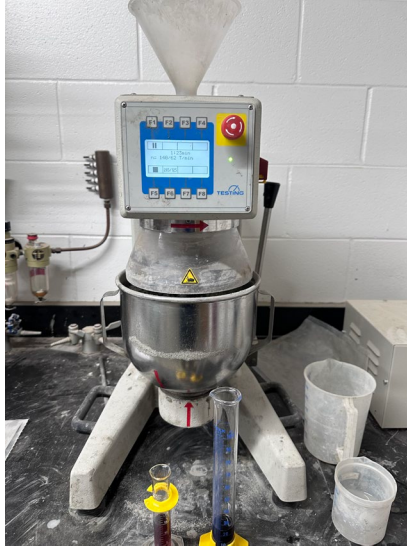
Figure 3-1 Planetary mixer used for small batch mixing.
