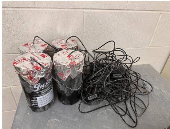
Figure 3-7 Cylinders with embedded wireless thermocouples monitoring internal concrete temperature profiles at early ages.
