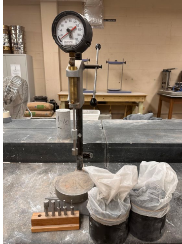
Figure 3-6 Setting time measurements with concrete penetrometer.
