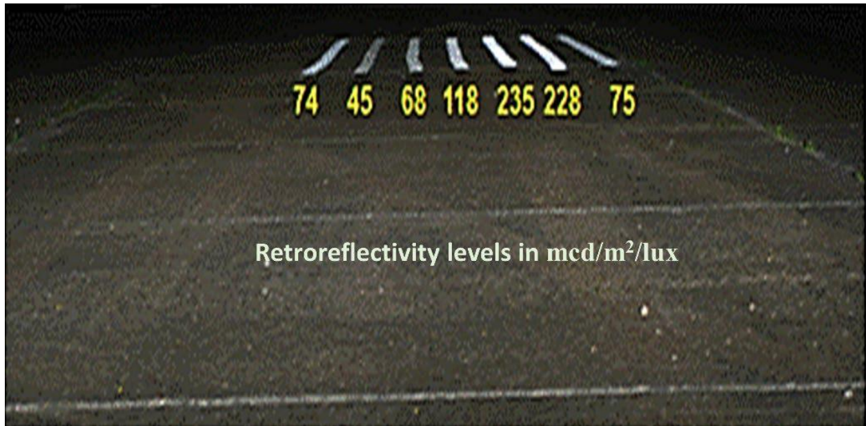
Figure 2 Pavement markings with different RL levels at nighttime (FHWA, 2017)
