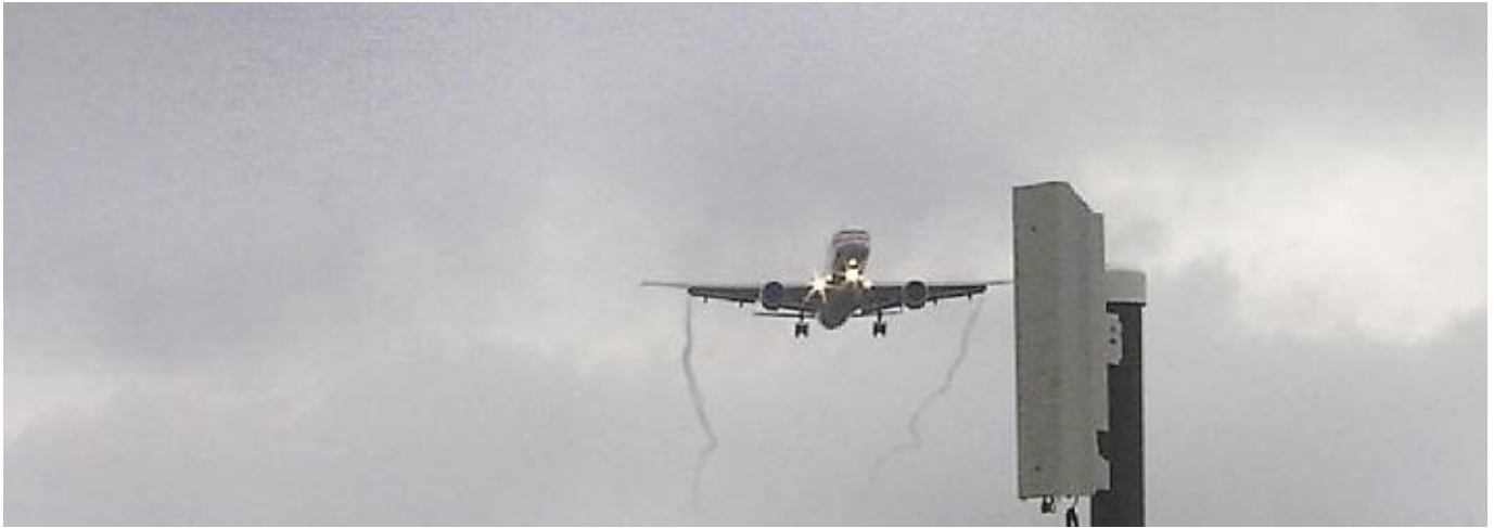
Volpe Center wake instrumentation during a landing at Lambert–St. Louis International Airport (STL). (Volpe Center photo)
