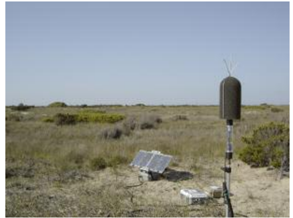
Noise measurement equipment gathers data for use by Volpe Center teams in developing acceptable and effective measures to mitigate or prevent significant adverse impacts from commercial air tours. (Volpe Center photo)
