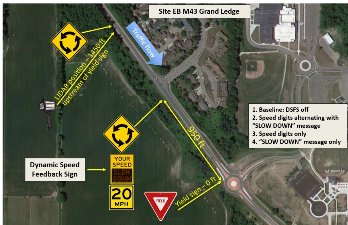
Figure 56. Field Evaluation Layout and Sign Test Conditions, EB M-43 Grand Ledge (Site 2)
