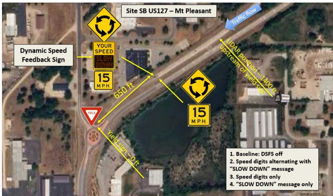
Figure 58. Field Evaluation Layout and Sign Test Conditions at SB US-127 Exit to Mt Pleasant (Site 4)
