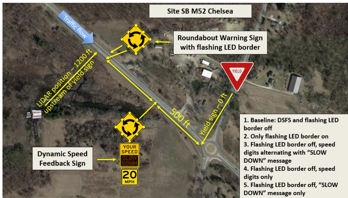
Figure 55. Field Evaluation Layout and Sign Test Conditions, SB M-52 Chelsea (Site 1)
