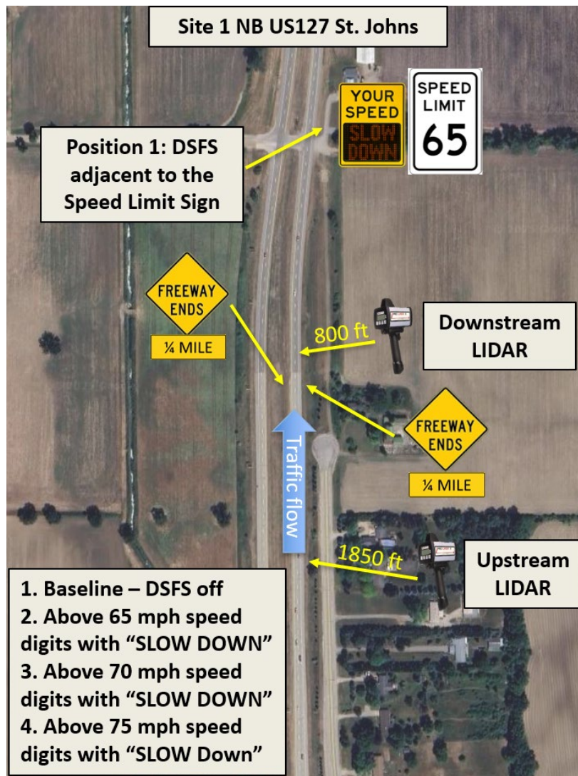
Figure 40. Field Layout and Sign Test Conditions at NB US-127 St. Johns, DSFS Position 2
