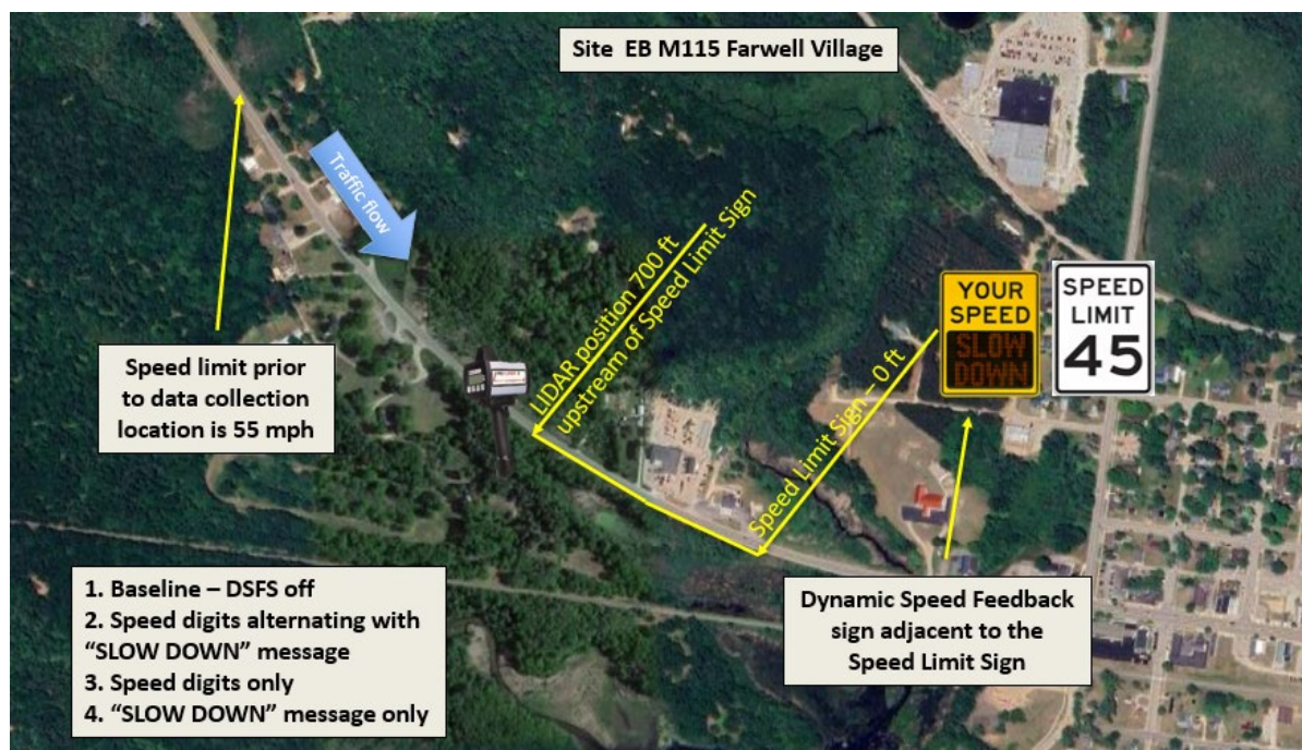
Figure 51. Field Evaluation Layout and Sign Test Conditions at EB M-115 Entering Farwell
