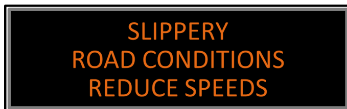
Figure 86. Recommended CMS Message for Winter Weather Warning at Bridge Overpasses
