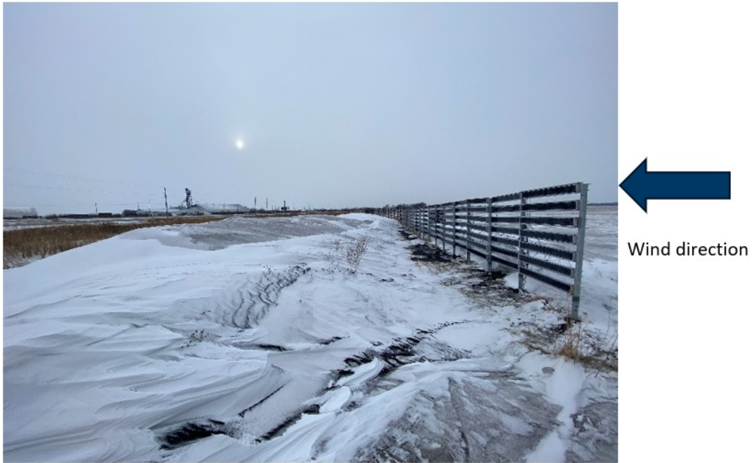
Figure 5.9 Comparison of the drifted snow between the solar snow fence and the traditional snow fence.
