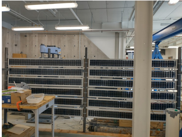
Figure 2.6 Front side of the prototype solar snow fence constructed in the Lab.
