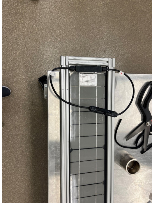
Figure 1.3 Assembled solar snow fence strip
