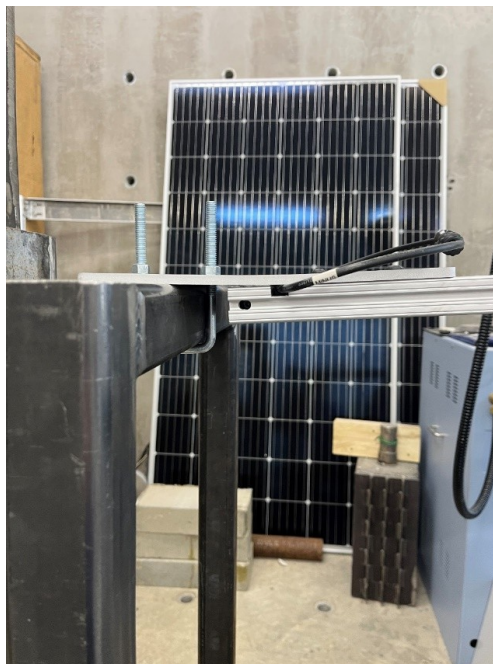
Figure 1.6 Front view of the designed connection under fatigue testing of a 30 psf wind load
