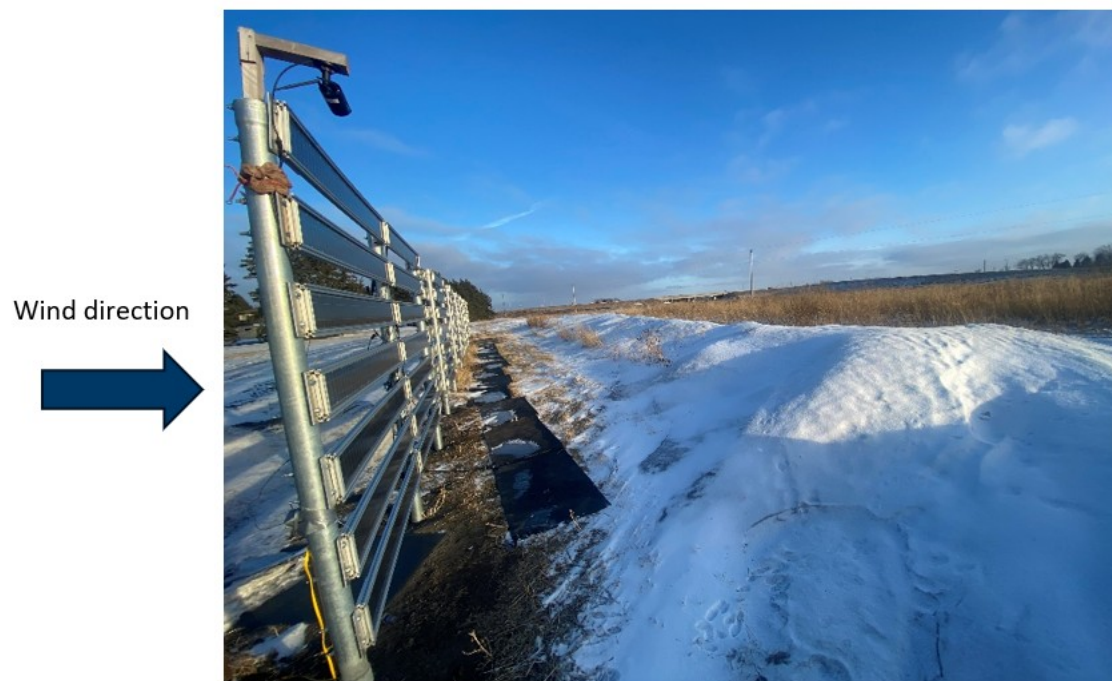
Figure 5.8 The melted gap formed by the solar snow fence.
