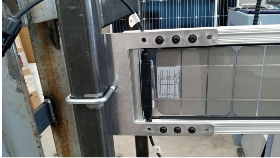
Figure 1.11 Zoom-in back view of the U-bolt connection in the vertical direction test setup
