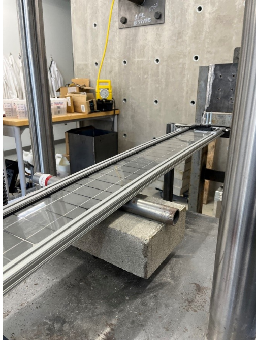
Figure 1.5 Front view of the designed connection under fatigue testing of a 30 psf wind load
