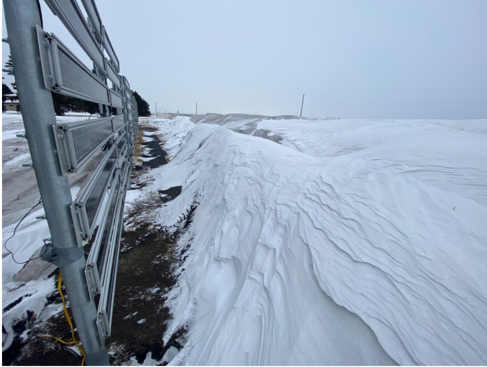
Figure 5.17 A close view of the snow melting pad and the drift profile formed in January 2025.
