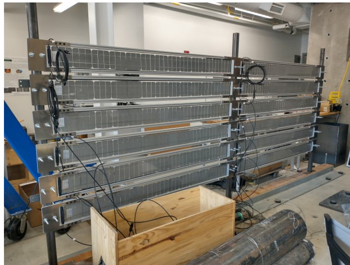
Figure 2.7 Back side of the prototype solar snow fence constructed in the Lab.
