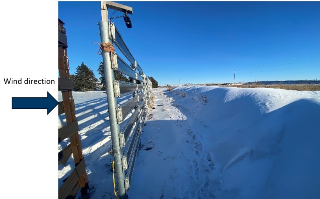
Figure 5.7 Drift snow profile formed by the solar snow fence with the snow melting pads.
