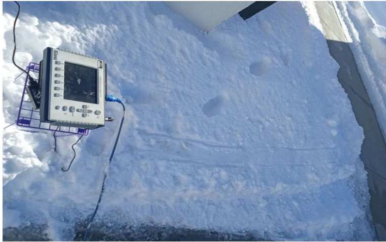
Figure 4.10 6-ft Snow strip used in the snow depth detection test.
