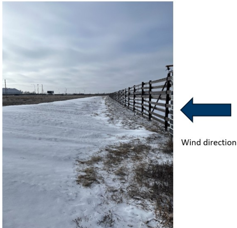
Figure 4.13 Comparison of leeward drift snow profiles formed by the solar snow fence and the traditional snow fence.
