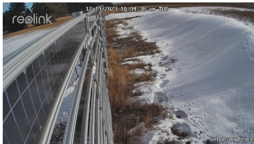
Figure 4.12 The drift snow profile formed by the solar snow fence implemented.
