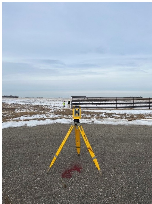
Figure 4.3 Recording of snow depth measurement locations using the GPS total station on Oct 15, 2022.
