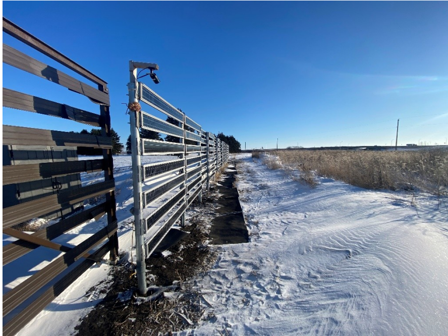
Figure 5.15 The clear walkway path formed by the 16 snow melting pads in October 2024.
