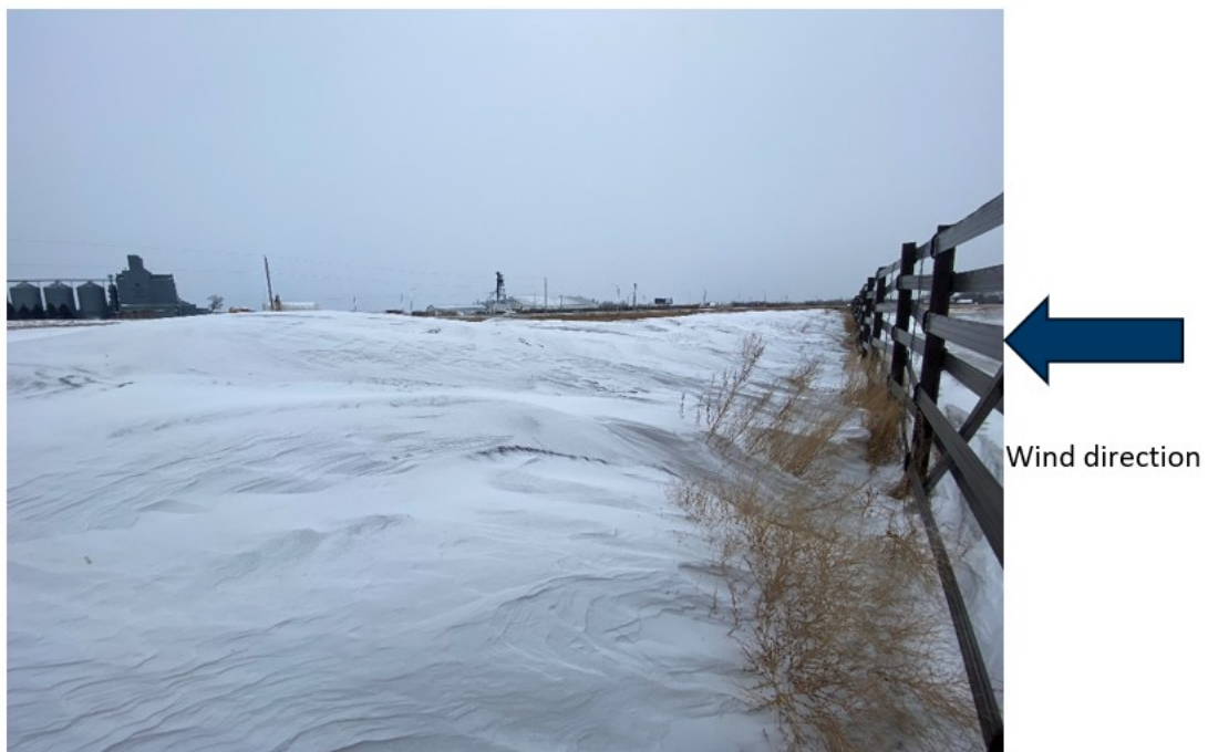
Figure 5.10 The drifted snow behind the traditional snow fence.
