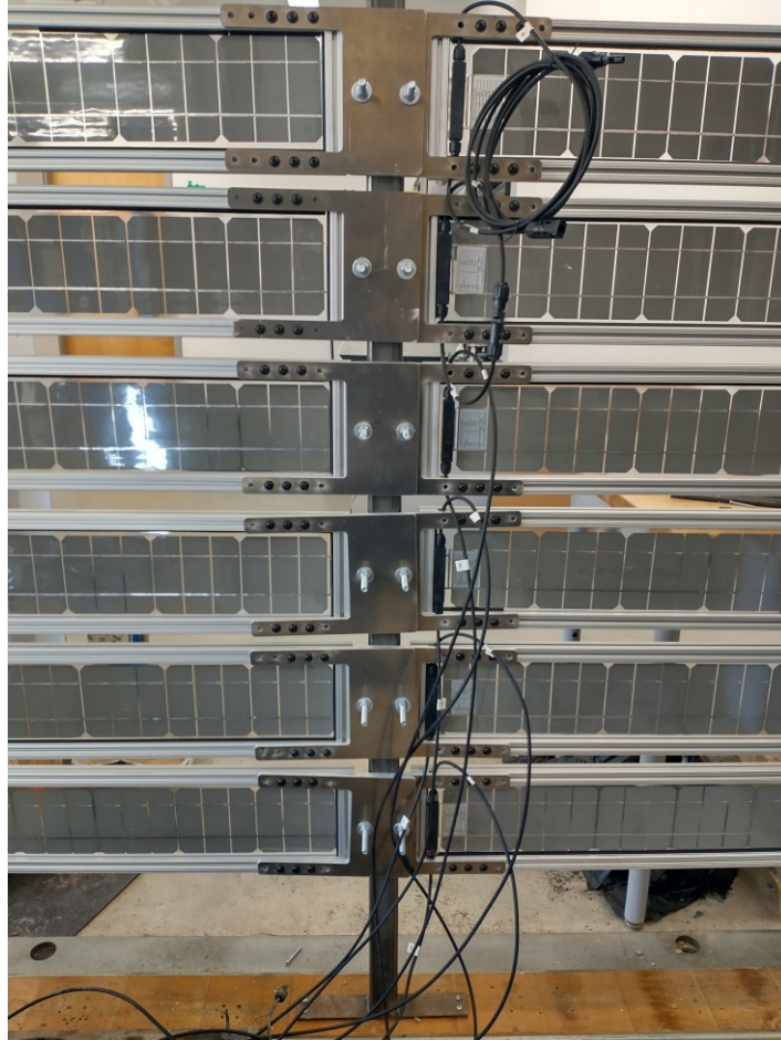
Figure 2.8 The back side U bolt connection adopted for the solar snow fence system.
