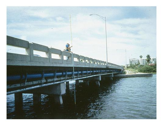
Figure 9.1 Sounding pole measurement.
