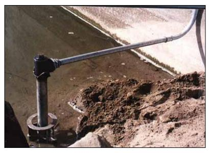
Figure 9.16. Detail of magnetic sliding collar on the streambed.
