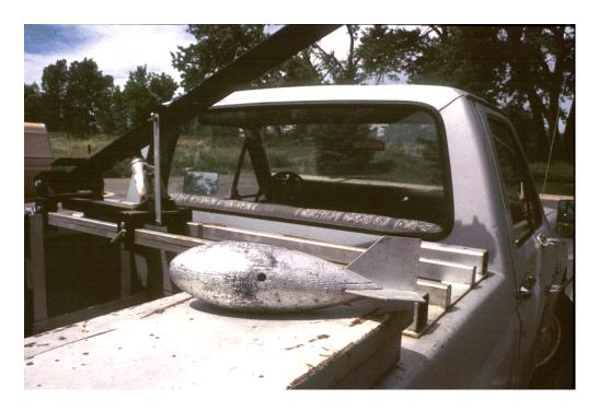
Figure 9.2. Lead-line sounding weight.
