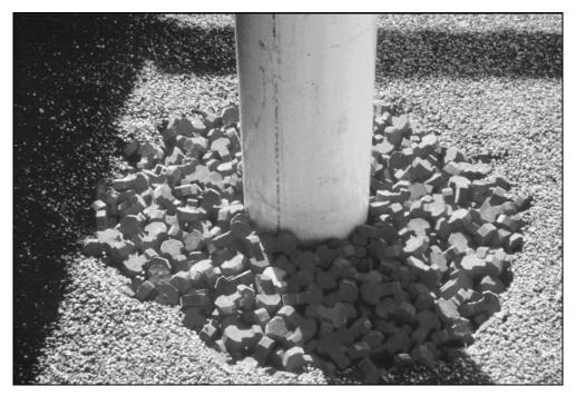
Figure 5.23. Laboratory study of Toskanes for pier scour protection.
