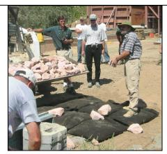
Demonstrating puncture resistance of geotextile containers
