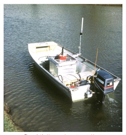
Figure 9.10. Unmanned, remote control boat.
