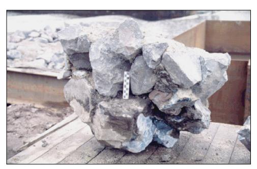
Figure 5.21. "Conglomerate" of partially grouted riprap, Federal Waterway Engineering and Research Institute, Karlsruhe, Germany (Heibaum 2000).
