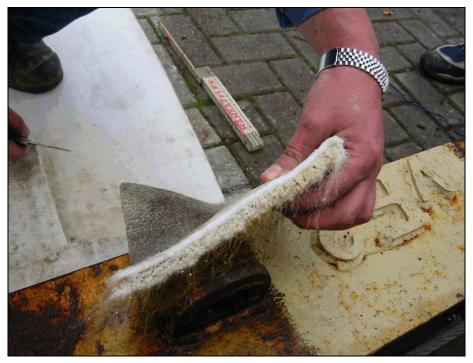
Figure 5.2. Close-up photo of SandMat<sup>TM</sup> geocomposite blanket. (photo from NCHRP Project 24-07(2), courtesy Colcrete – Von Essen Inc.)
