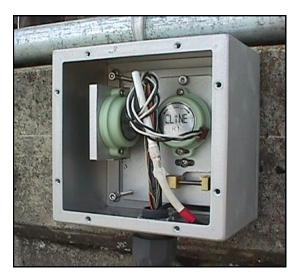
Figure 9.19. Detail of tilt meter.
