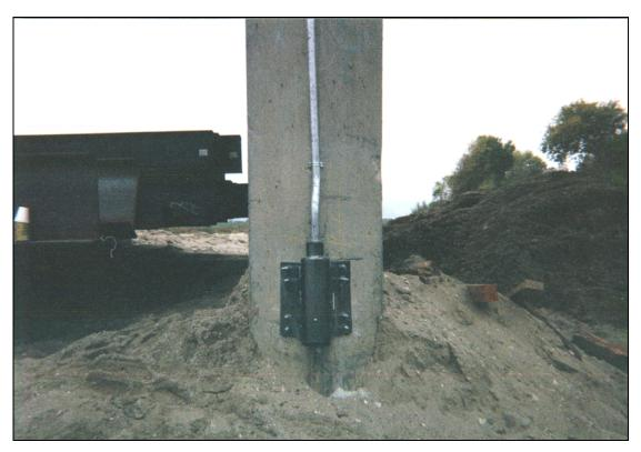
Figure 9.28. Close up of sonar scour monitor on Salinas River Bridge near Soledad, CA.
