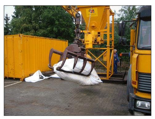
Figure 5.6. Handling a 1.0 metric tonne sand-filled geotextile container. (photo from NCHRP Project 24-07(2), courtesy Colcrete – Von Essen Inc.)
