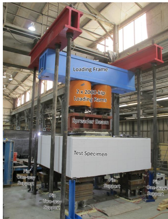
Figure 3-80. Test setup for drilled shaft footing specimens
