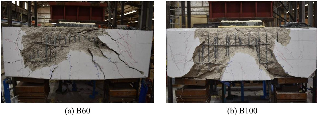
Figure 3-84. Deformed side face reinforcement after failure
