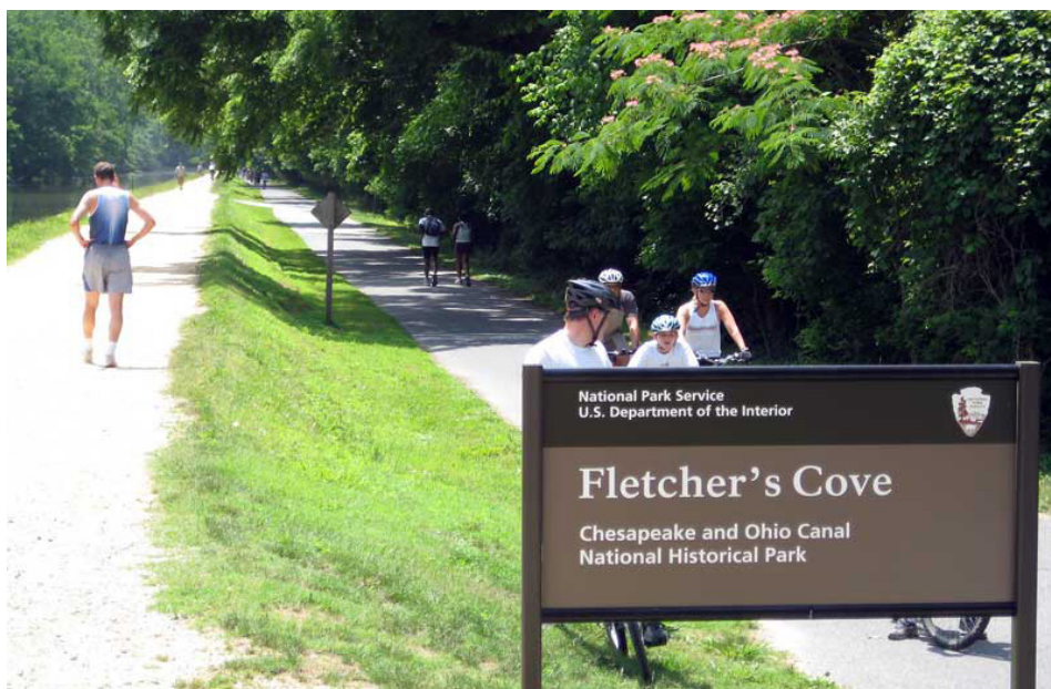
Figure 3-16: A multiuse trail at Chesapeake and Ohio Canal National Historical Park in Washington, D.C. includes a gravel path and a parallel paved path to provide options for pedestrians, bicyclists, runners, and others using the trail. (Source: National Trails Training Partnership) 20
