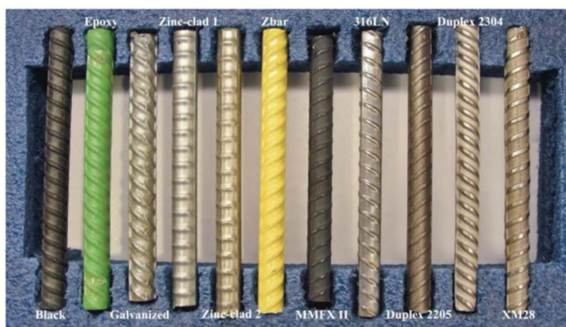
Figure 2.7 Corrosion-resistant steel evaluated (Sim, 2014).
