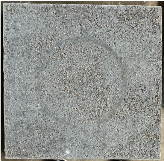
Figure 6.6: Aggregate embedment and loss on Broadcast Calcined Bauxite Lo-w/c sample (a) after brushing, (b) after conditioning, (c) after DFT testing
