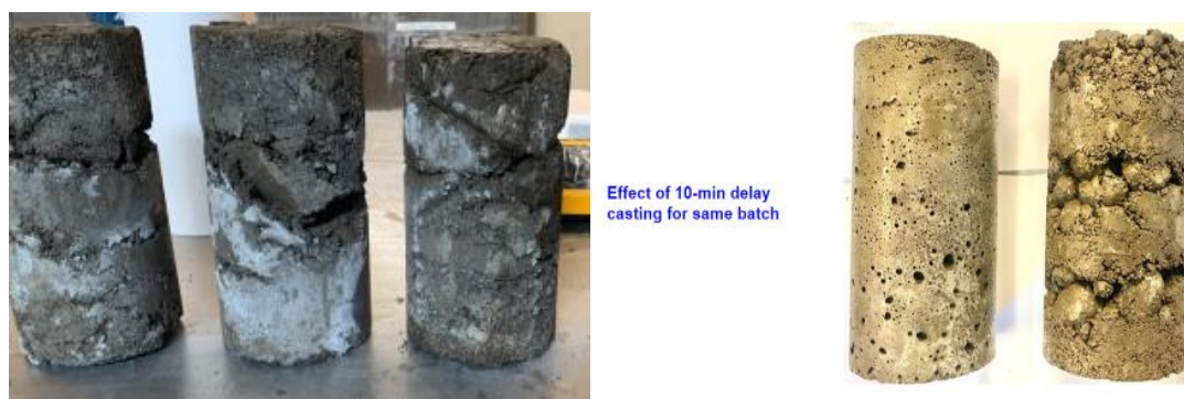
Figure 17: Influence of Elevated Temperature on RSPM Casting
