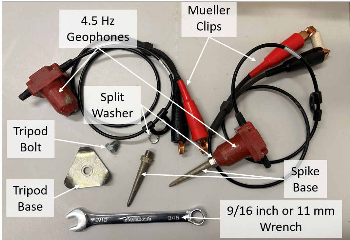
Photograph of 4.5-Hertz Vertical Geophone Setup.
