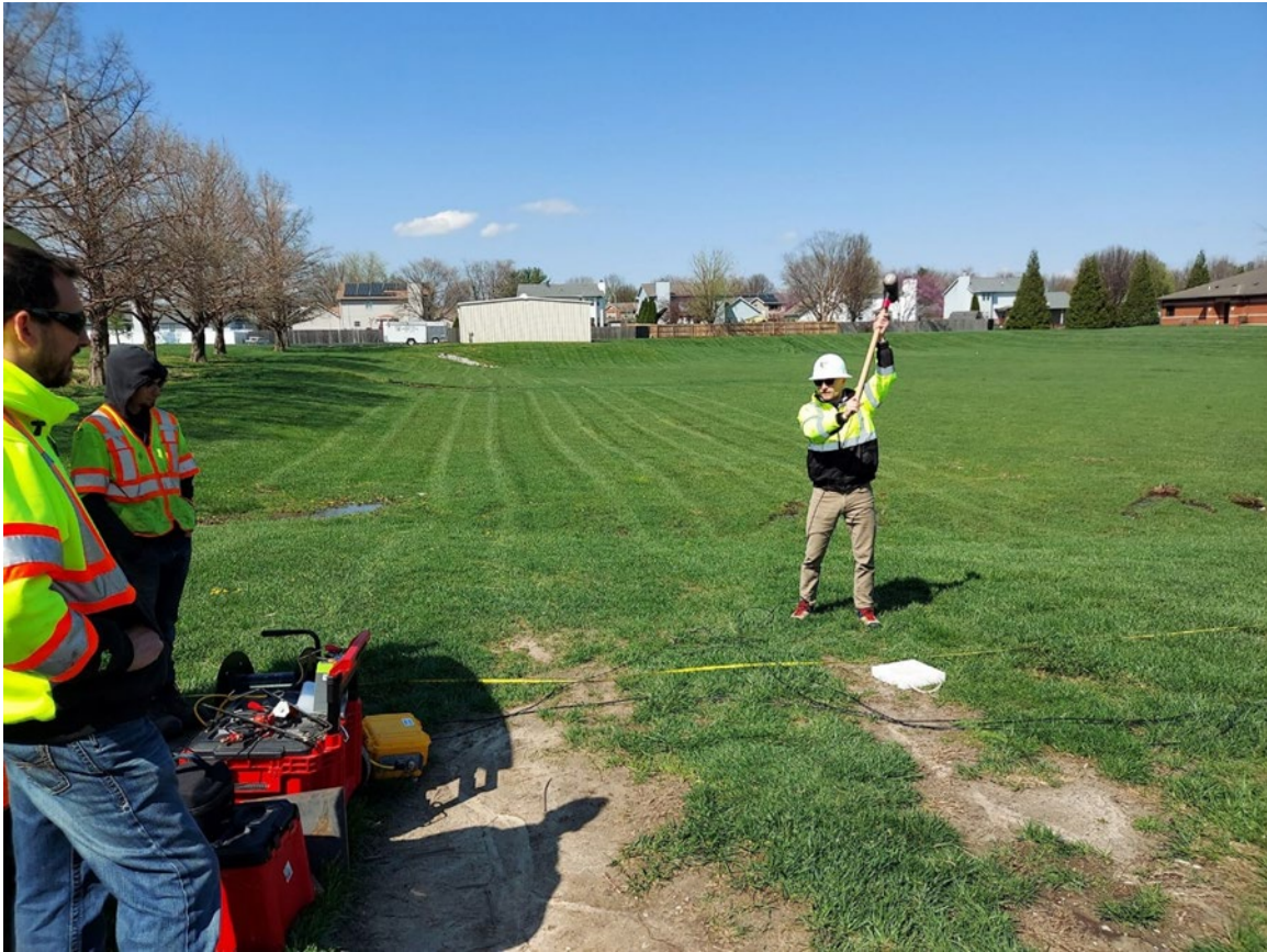
Photograph of a field staff member prepared to generate acoustic energy for an Active data survey by striking the plate with a 20-pound sledgehammer.
