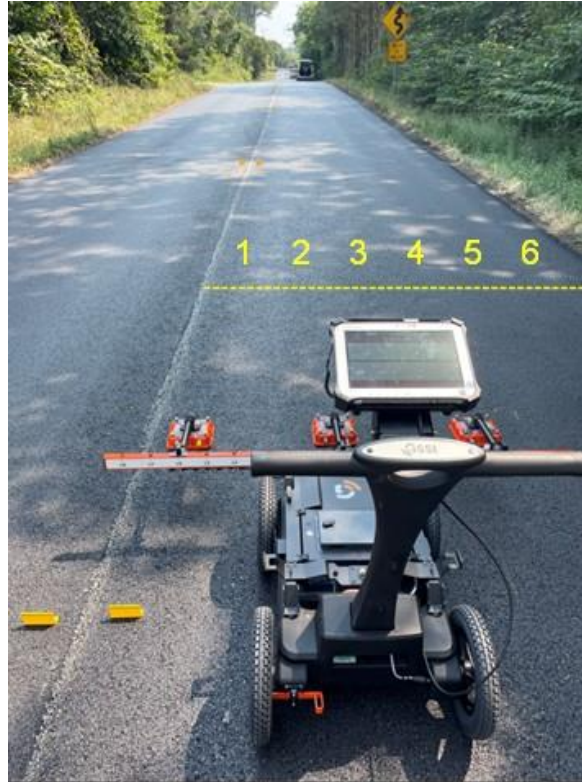
Figure 3. Density Profiling System Field Testing Showing Six Antenna Passes per Lane
