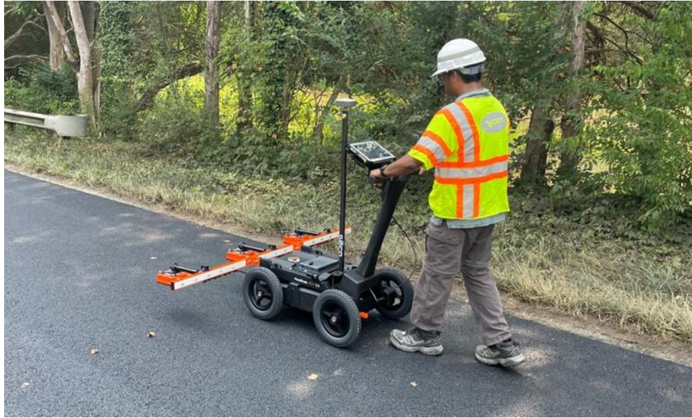
Figure 1. Field-Based Density Profiling System
