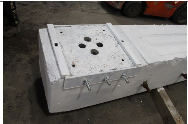
Shear-key details with steel plates and anchors
