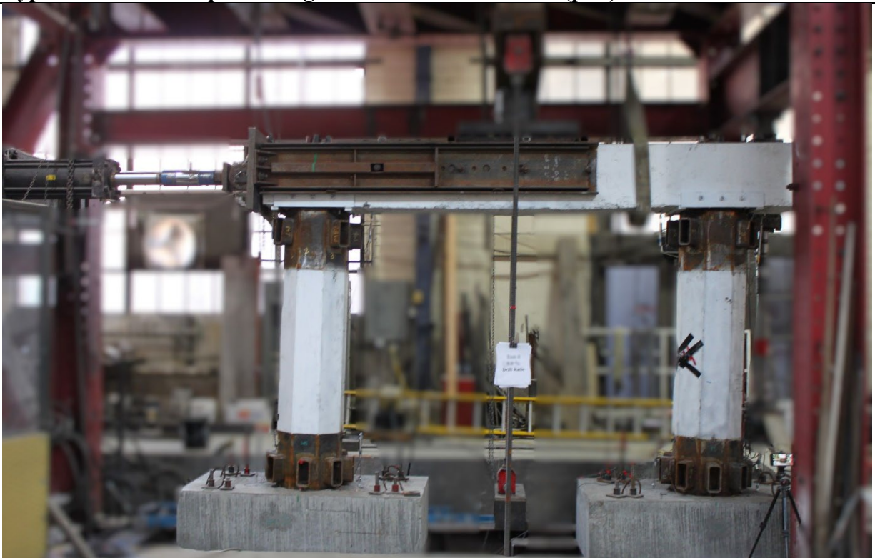
Typical deflected shape of bridge bent at 4.0% drift ratio (push)
