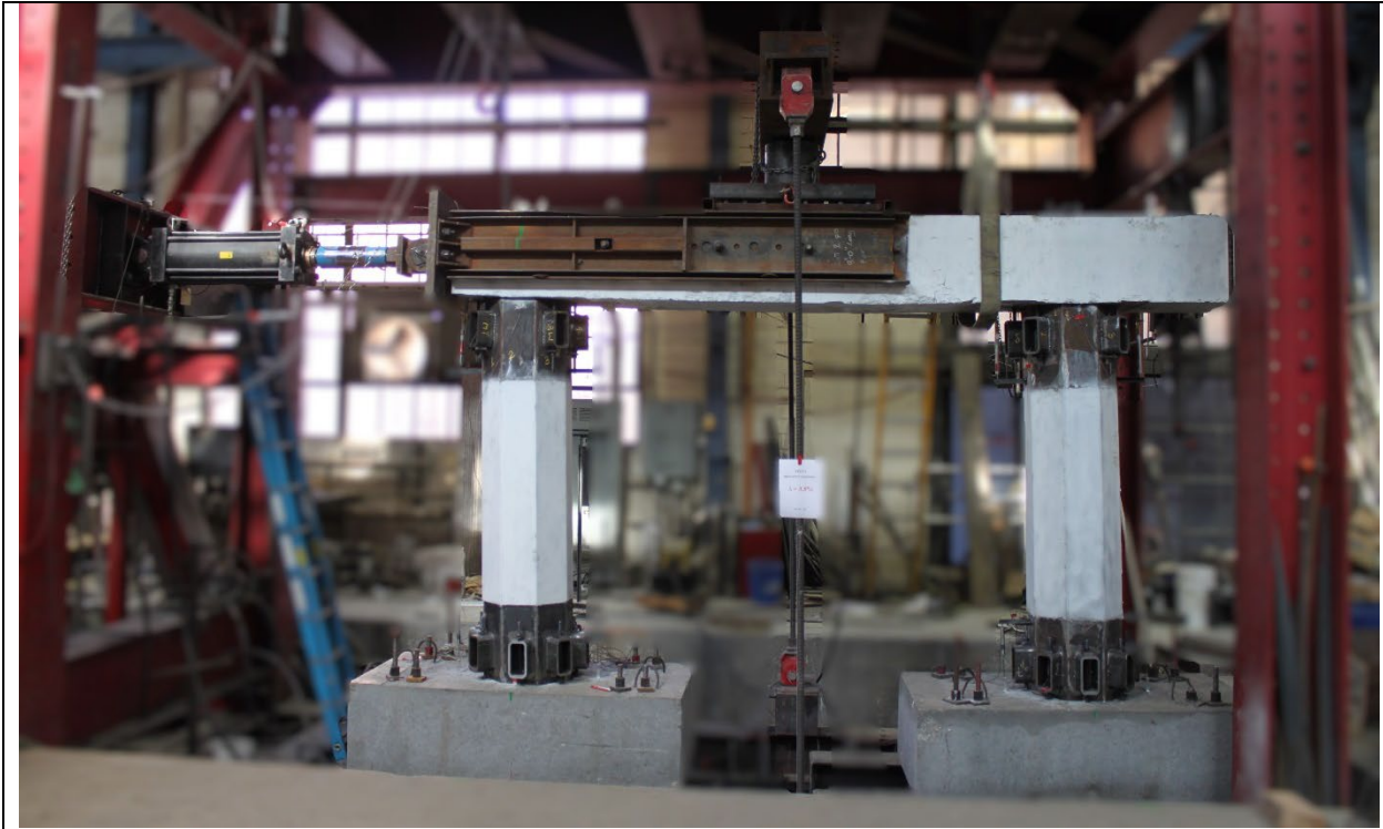
Typical deflected shape of bridge bent at 3.5% drift ratio (pull)
