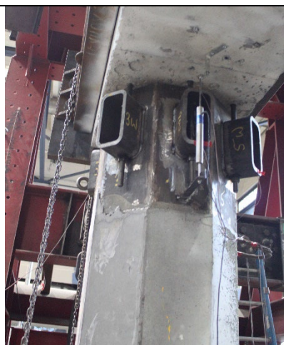
LVDT at cap-beam
