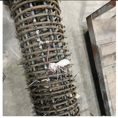
Strain gauges attached to column reinforcement cage
