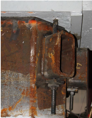
SLA elongation (cap-beam)
