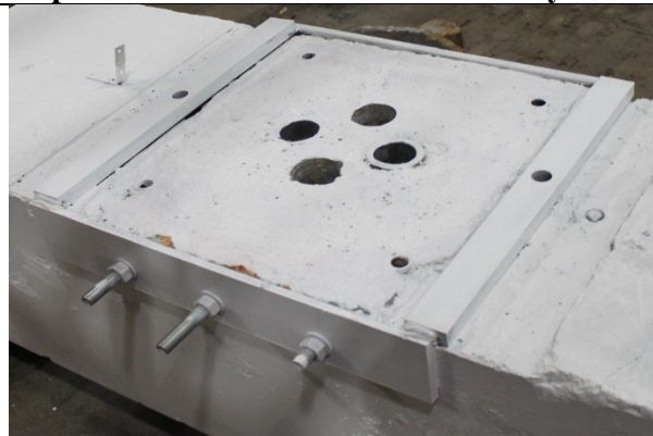
Shear-key details with steel plates and anchors
