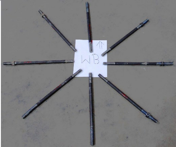
SLAs after test (West column footing SLAs)
