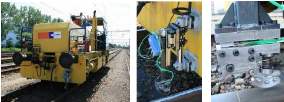
Fig. 5.8 Rolling stock and Sensor mounted.
