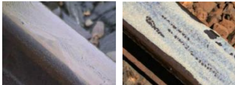
Fig. 5.9 Contaminants applied on the track: KajoBio (left) and Sandite (right).
