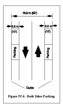
The number of through lanes and the lane width should be coded according to the striping, if present, on multilane facilities, or according to the traffic use if no striping or only centerline striping is present. For example, the number of through lanes in Figure IV-6 would probably be 2 and the lane width might be 3.9 meters (13 feet), even though 5.3 meters (17.5 feet) are available, since traffic would normally only use the middle portion of the roadway.
