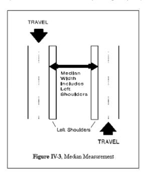
Enter the predominant median width (including left shoulders, if any; see Figure IV-3), measured between the inside edges of the through roadways, to a tenth of a meter (xx.x -- implied decimal) or the nearest foot. Enter "000" for undivided or nonapplicable roadways. Enter "999" where the median width is 100.0 meters or 1,000 feet or greater. Provide leading zeroes if applicable. Ignore turning bays cut into the median.
