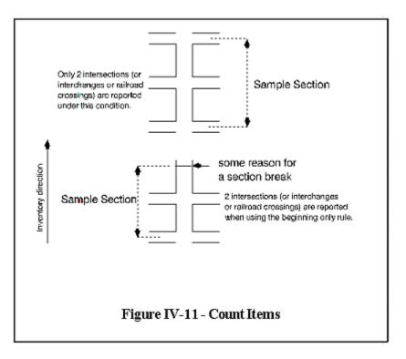
In the upper portion of Figure IV-11, the intersection count would always be two regardless of the inventory direction or the beginning/ending only rule. There may be differences in other data items, however, since items such as green time, turning lanes, etc., would depend on what rule the State is using. For example, if the State always counts the beginning only, the ending intersection would be ignored for all data items affected by intersections.
