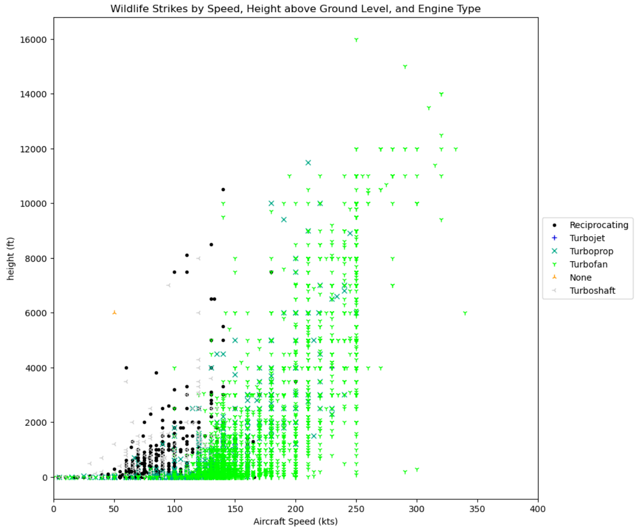
Figure 42. Wildlife strikes based on speed, height, and engine-type (n = 8,064, one strike at around 650 kts excluded)
