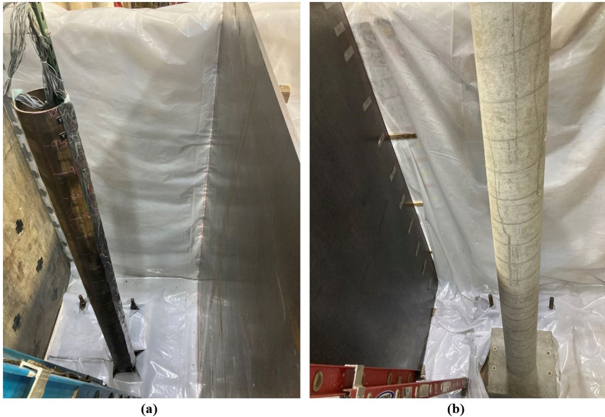
Figure 4.13. Specimen before filling of Type B TDA (a) Specimen QS01, and (b) Specimen QS04.
