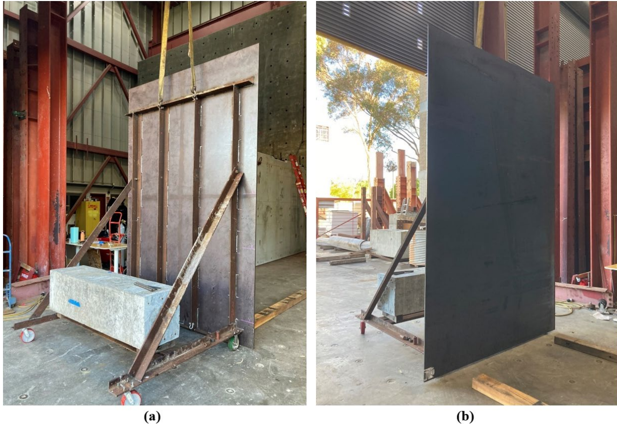
Figure 4.12. Moving wall and truss support: (a) Front side and (b) Back side.
