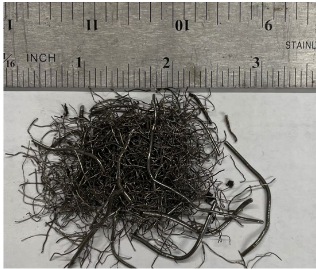
Figure 5.8: Sample of COR-TUF UHPC recycled steel fibers.
