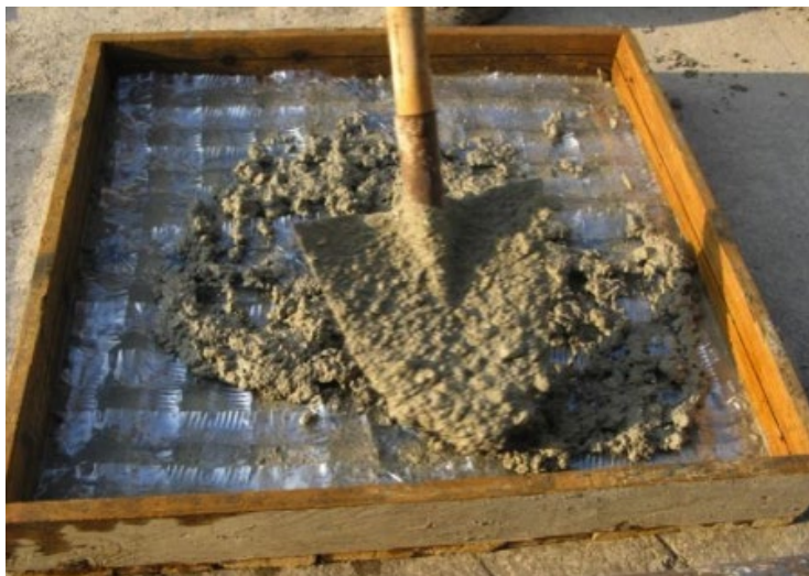
Figure 3.2: Concrete cast over an rPET grid.
