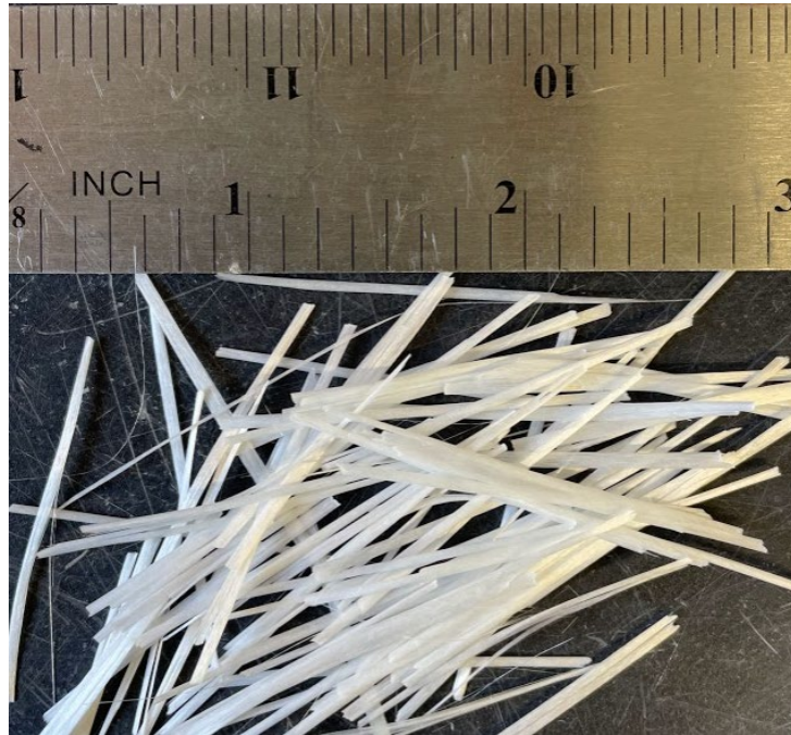
Figure 7.4: A picture of a sample of Anti-CRAK HP 67/36 silica glass fibers.
