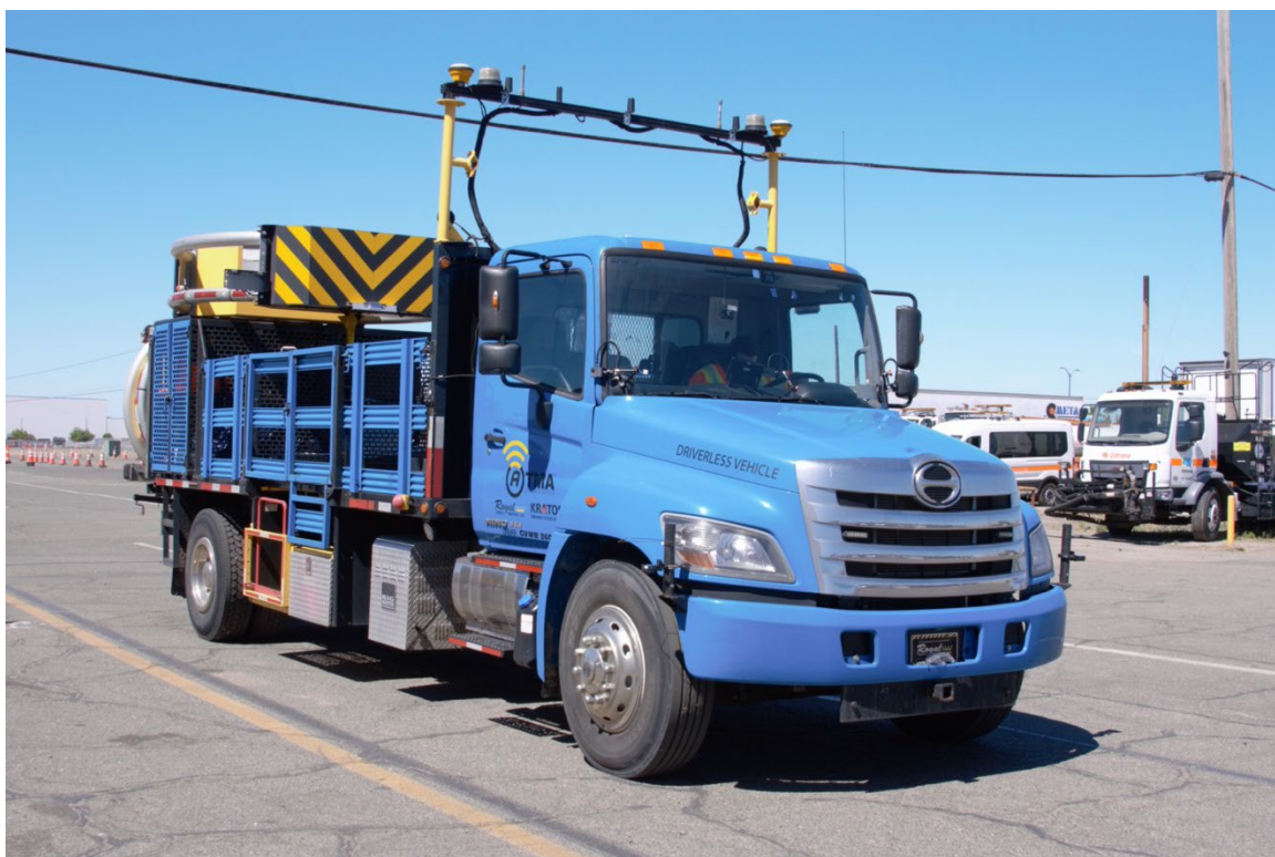
Figure 4.5: Side view of the RCTMA equipped with all sensors
