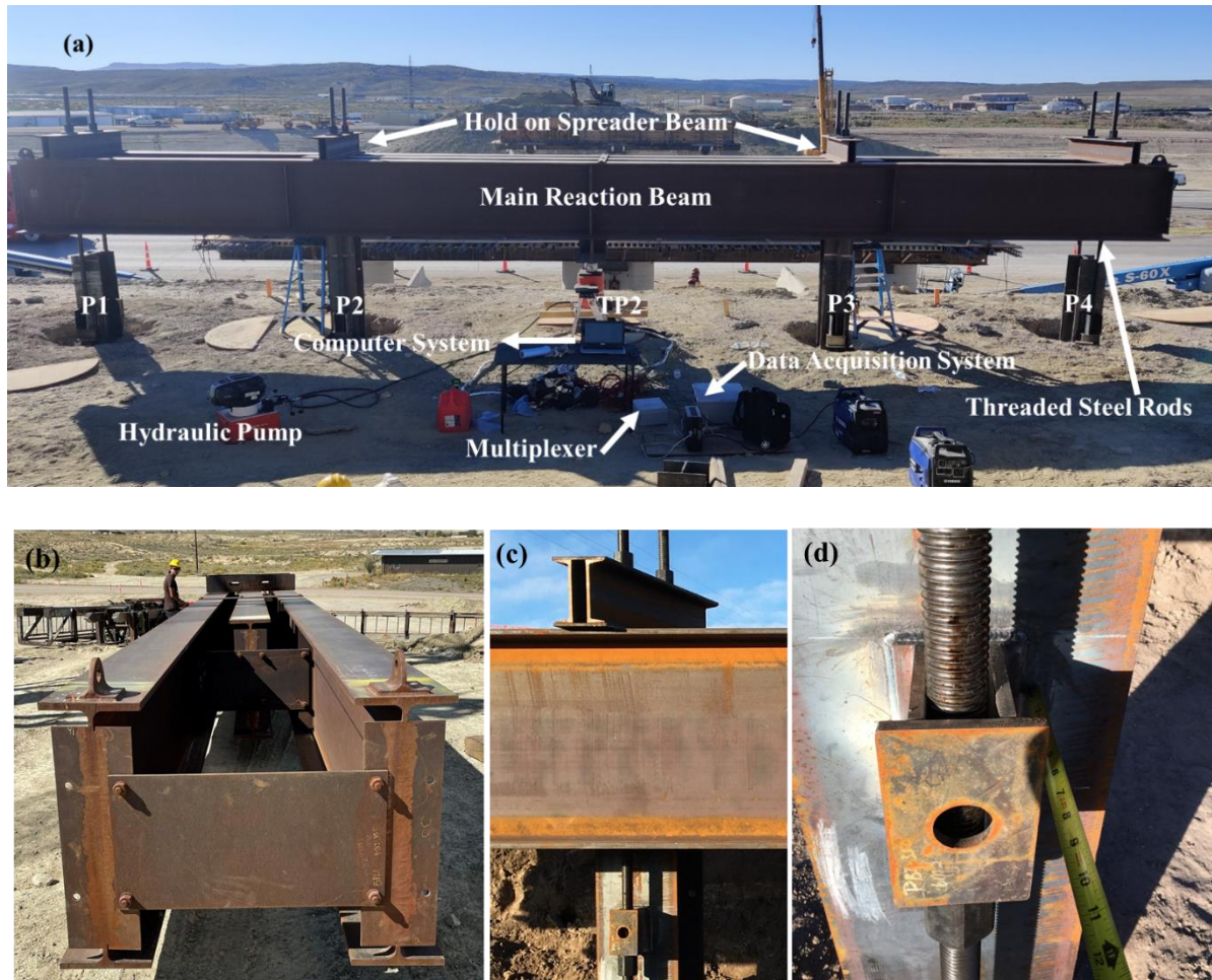
Figure 3.3. Static Pile Load System: a) InteSPLS on TP7 in Sweetwater County, WY, b) Main Reaction Beam System, c) Assembly of Spreader Beam, Main Reaction and 1.75-in Diameter HS Treated Bar, and d) A Treated Bar and Anchor Block of the InteSPLS.
