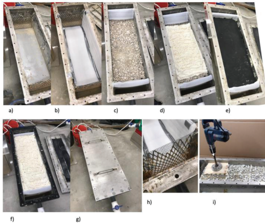
Figure 5.4 (a–g) Preparation of compacted sample in large permeameter; (h) detail of screens at ends of permeameter; and (i) compaction of last aggregate lift with vibratory hammer on wooden pad.
