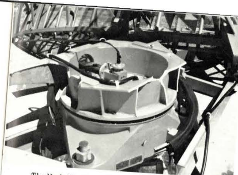
The Nashville, Tenn., ASR and SECRA antennas lie beyond the broken pedestal, looking more like plastic than steel.
