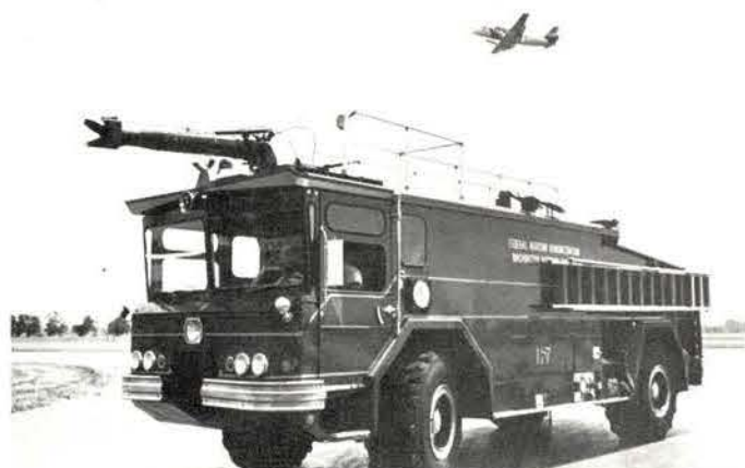
Lt. Albert Coe and driver James Pete roll a crash truck into action. It carries 3,000 gallons of water and 500 gallons of chemical foam and can be serviced by a tanker truck.
