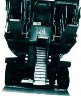
The business end of a conventional mobile lounge with its staircase unfolded. It can serve for easy access of flight crews to the ground.
