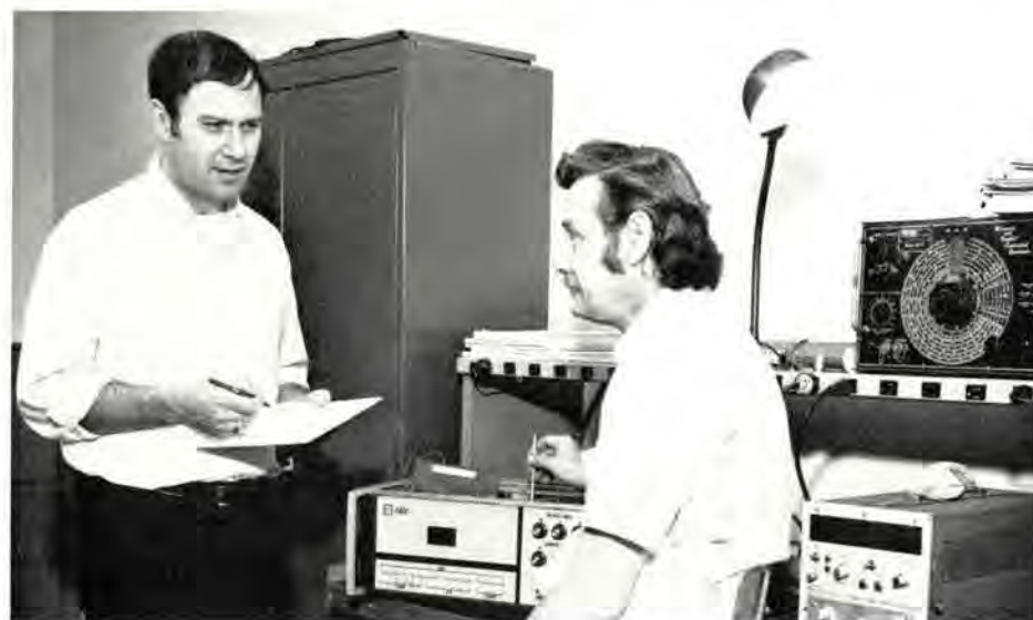
Joe Dillon (left) and Walt Threewitt, Great Lakes AF engineers, check over the prototype of their energy demand control computer, which not only conserves energy but money for commercial users, which savings could be passed on to the consumer. Newer models provide a chart readout for studying and monitoring electricity usage.
