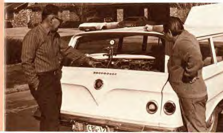
Bill Goldsberry (left) shows Amarillo Tower chief J. V. Vinyard the 20 tanks for natural gas storage in the back of his station wagon. A tarp is used to cover them.
