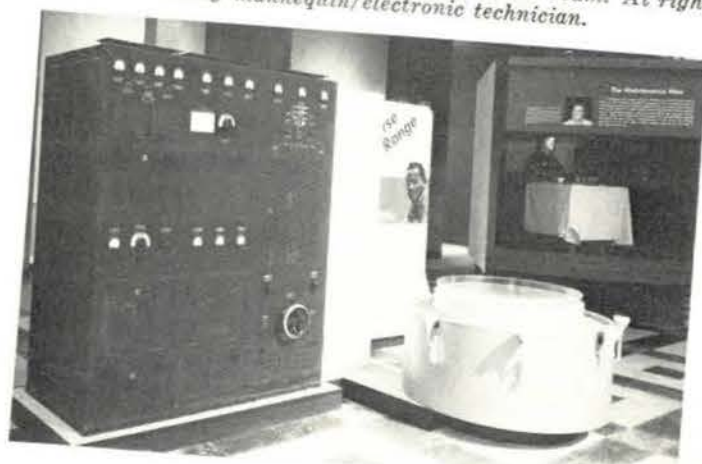
This Four-Course Radio Range transmitter was commissioned in 1936 in Daggett, Calif. Pilots rode in on its beam. At right rear is a talking mannequin/electronic technician.
