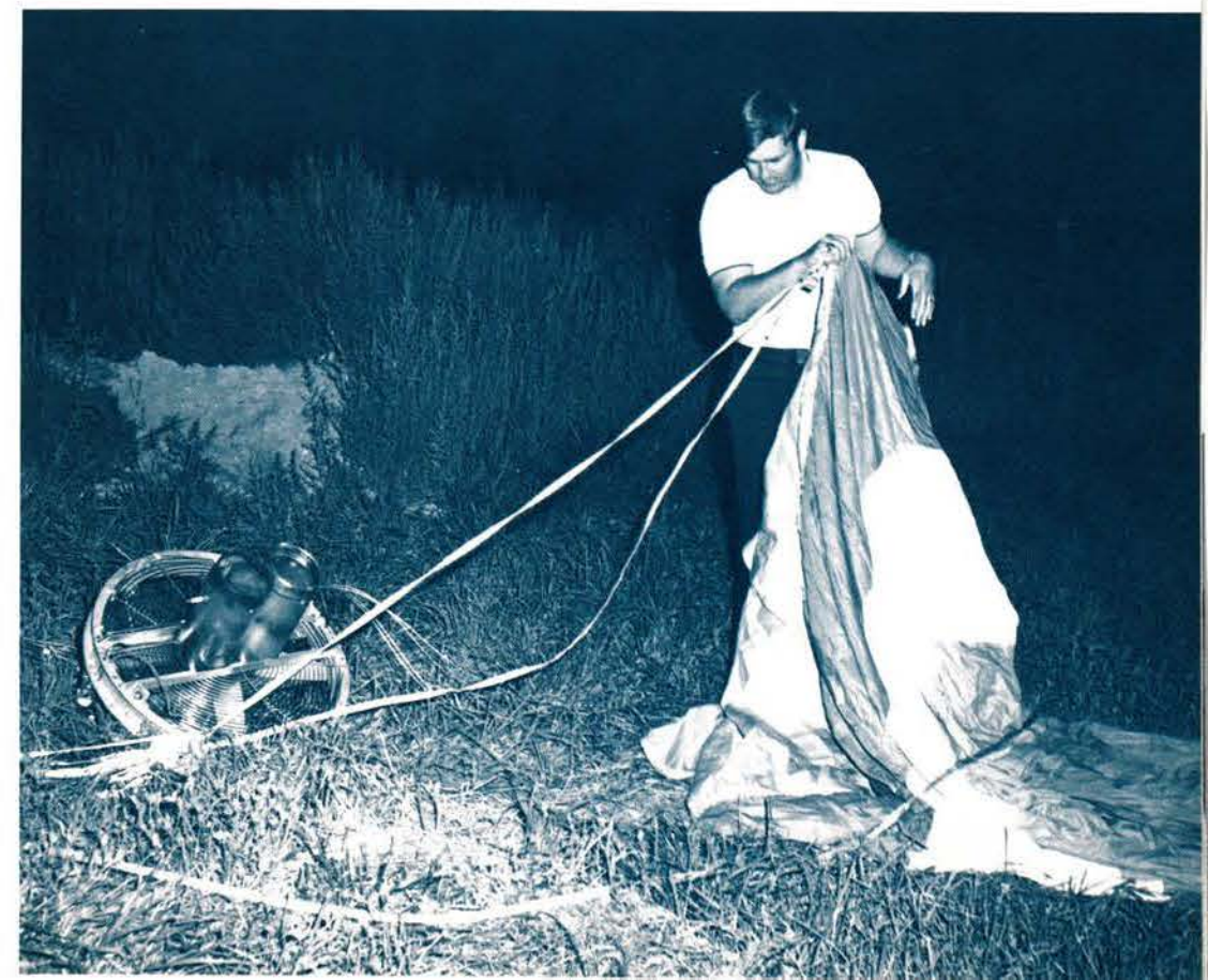
Ward sorts out the cables for hooking the burner and fan to the balloon. Assembly and inflation takes a total of 45 minutes.
