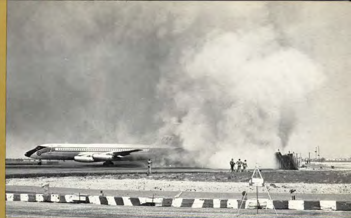
BLAST NO MORE —With NAFEC test pilot Joseph Bailey at the controls, a Convair 880 runs up to full power at JFK Airport to test the effectiveness of a blast fence protecting another runway behind and perpendicular to it. The smoke is deliberate to outline the jet blast.
